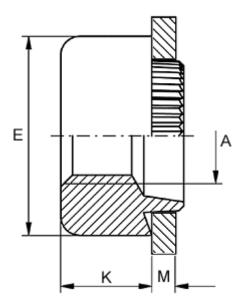
Female thread A = M6Height K = 5.0Outer diameter E = 10.0Plate thickness = 1.1 to 1.3
